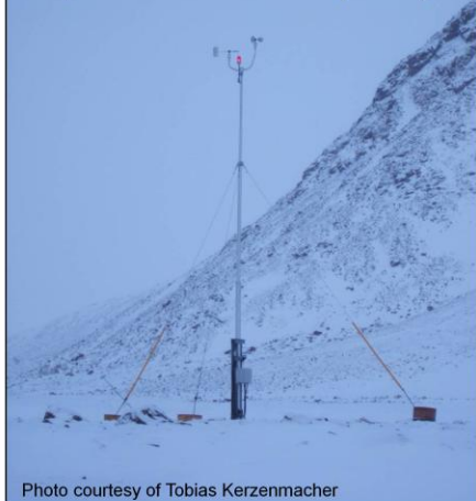
Anemometer (measures wind speed)
