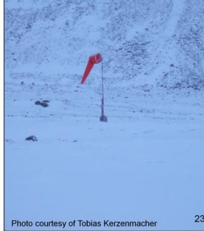
Wind Sock (measures wind direction)
