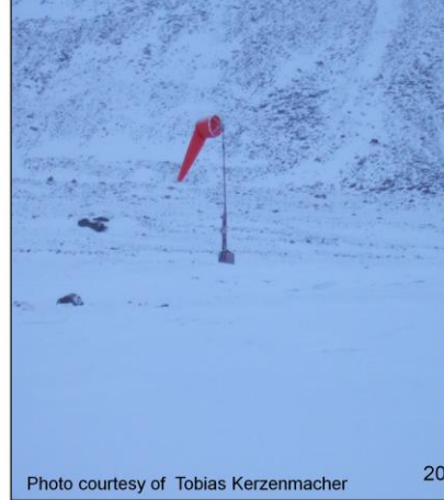
Wind Sock (measures wind direction)
