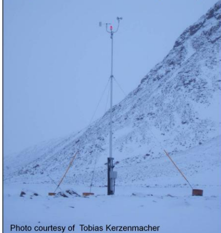
Anemometer (measures wind speed)
